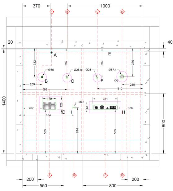
Figure A1.1: Elevation of Test Specimen, Unexposed side
