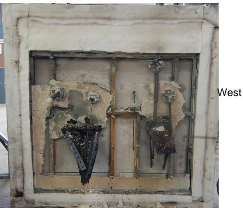
Figure A6.4: Exposed face of specimen at the end of the test.
