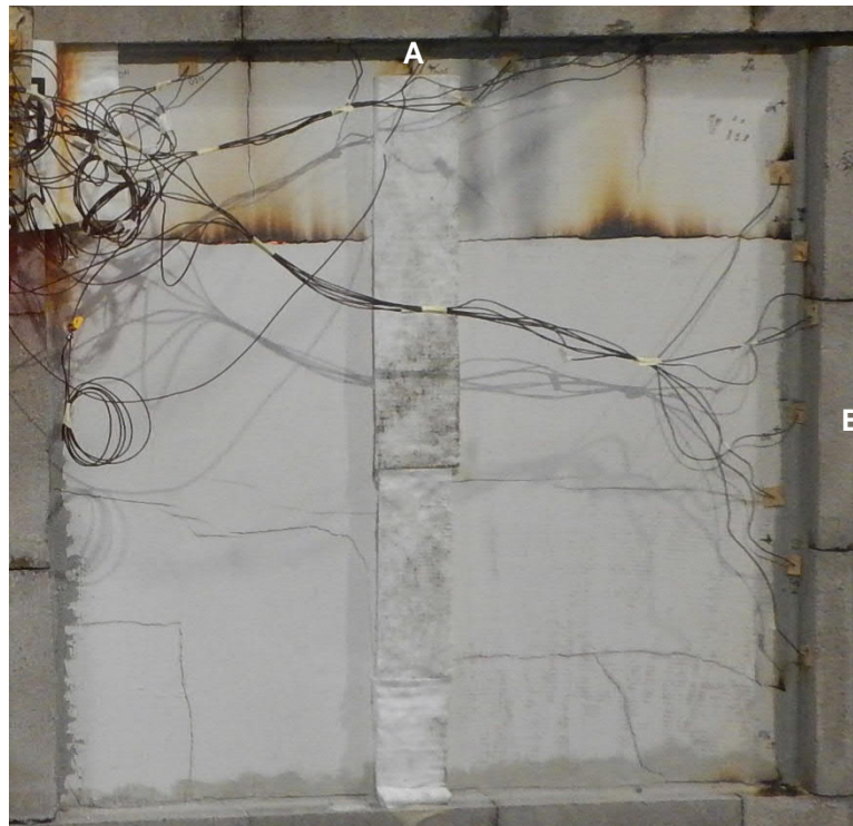
Figure 19 Unexposed face of the specimen at the end of the test
