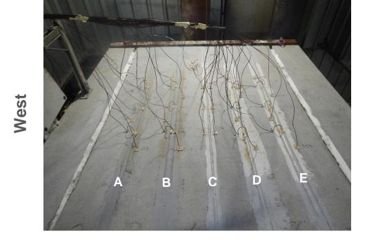
Figure 14 Unexposed face of the specimen at the end of the test
