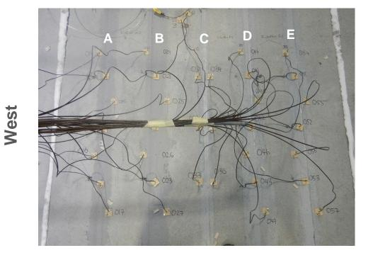
Figure 12 Unexposed face of the specimen before the start of the test
