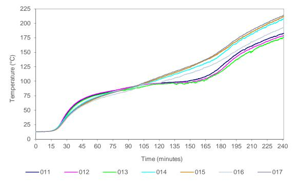
Figure 7 Control joint A- temperature vs time
