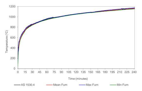
Figure 5 Furnace thermocouple temperature vs time
