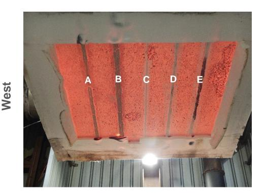
Figure 15 Exposed face of the specimen at the end of the test
