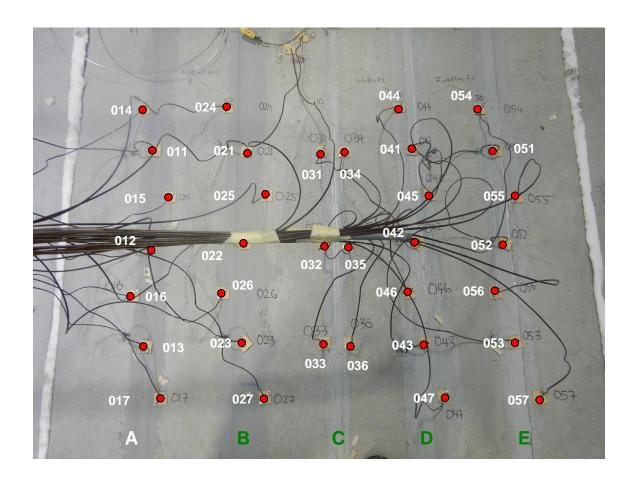
Figure 4 Unexposed side thermocouples
