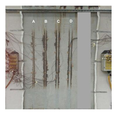
Figure 18 Unexposed face of specimen at the end of the fire-resistance test
