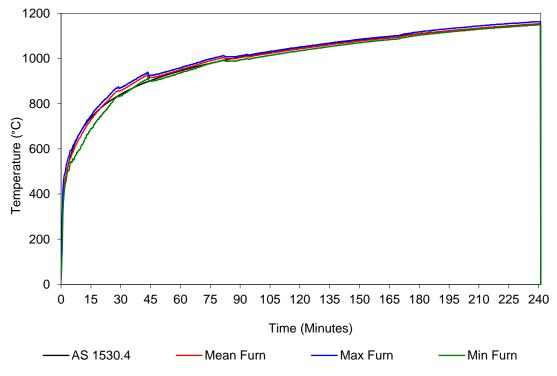
Figure 7 Furnace thermocouple temperature vs time
