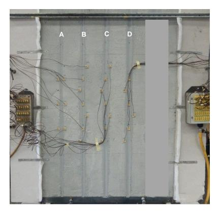
Figure 16 Unexposed face of specimen before the start of the fire-resistance test
