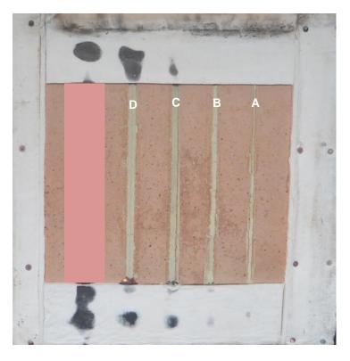
Figure 19 Exposed face of the specimen at the end of the fire-resistance test
