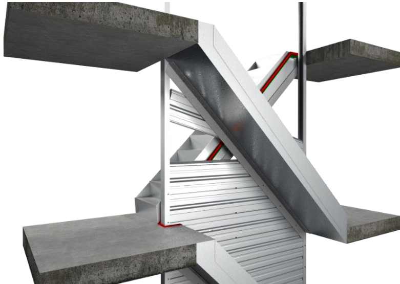
Figure 2 Single 78 mm thick horizontally stacked wall – steel angle at bottom of stringer
