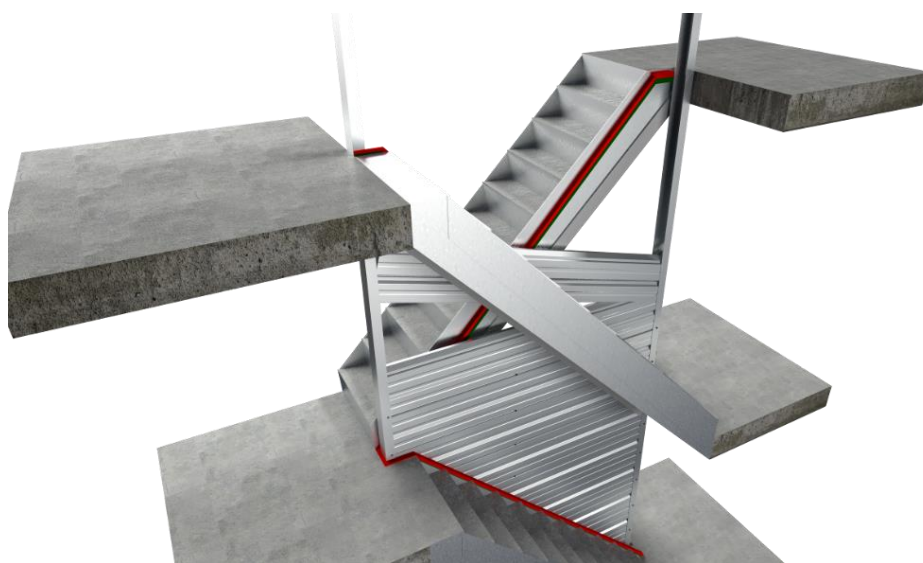
Figure 1 Single 78 mm thick horizontally stacked wall – Fuller Firesound Acrylic Sealant shown in red
