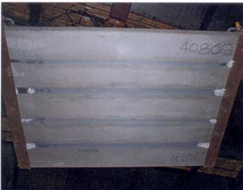
Plate 2: Exposed face before commencement of the fire resistance test
