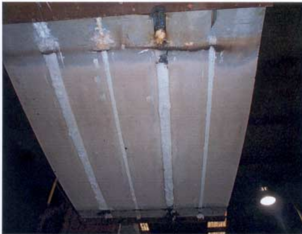
Plate 4: Exposed face after completion of the fire resistance test
