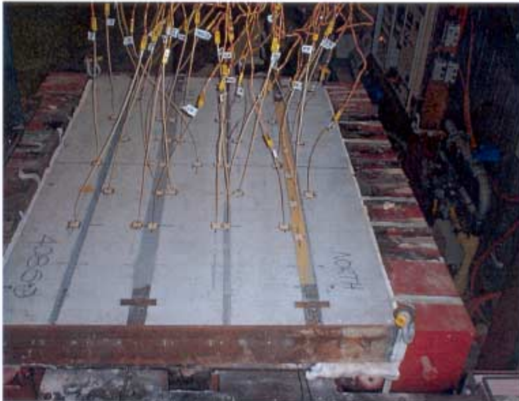
Plate 1: Unexposed face before commencement of the fire resistance test
