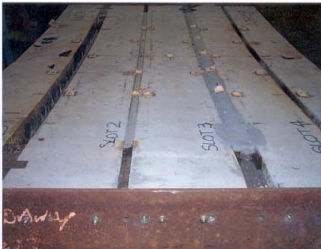
Plate 3: Unexposed face after completion of the fire resistance test
