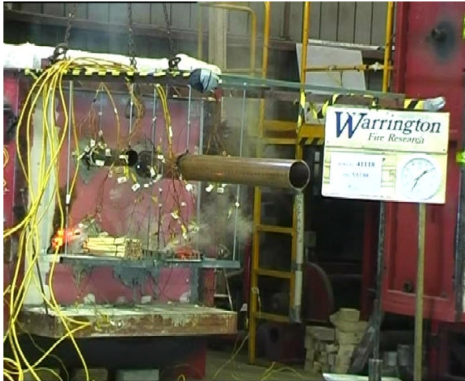
Plate 3: Partition failed integrity in accordance with AS 1530.4 -1997 at 98 mins by evidence of a through gap into the furnace.
