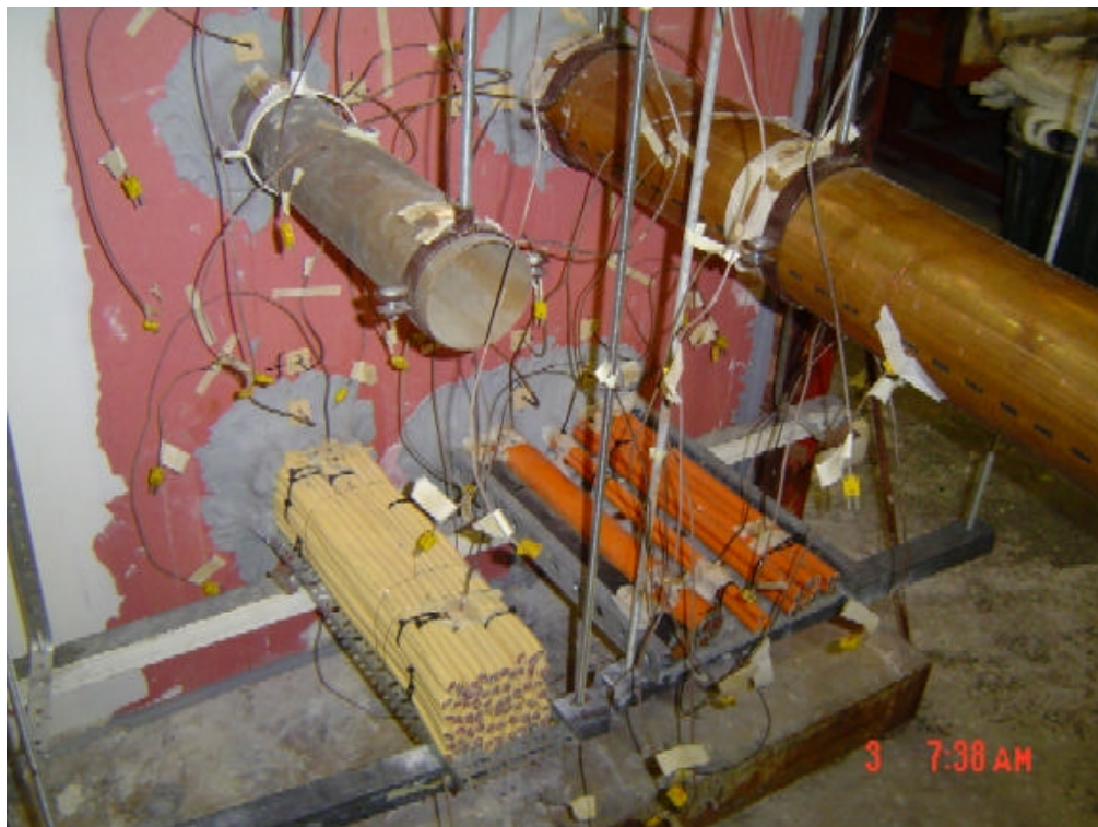
Plate 2: Unexposed face of test specimen prior to commencement of the fire-resistance test
