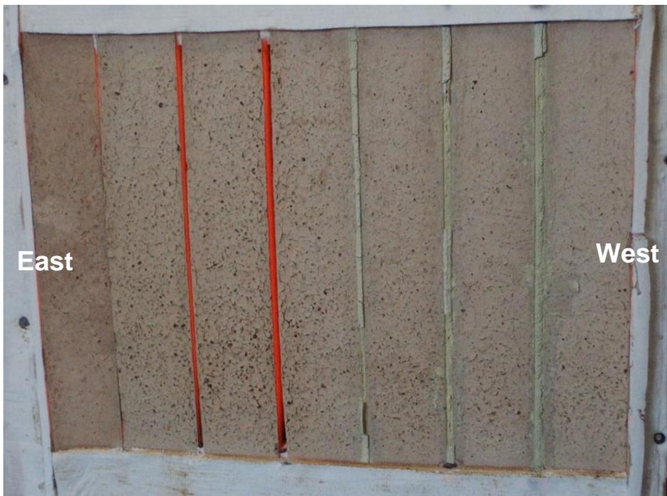
Figure 26 Exposed face of the specimen at the end of the fire-resistance test
