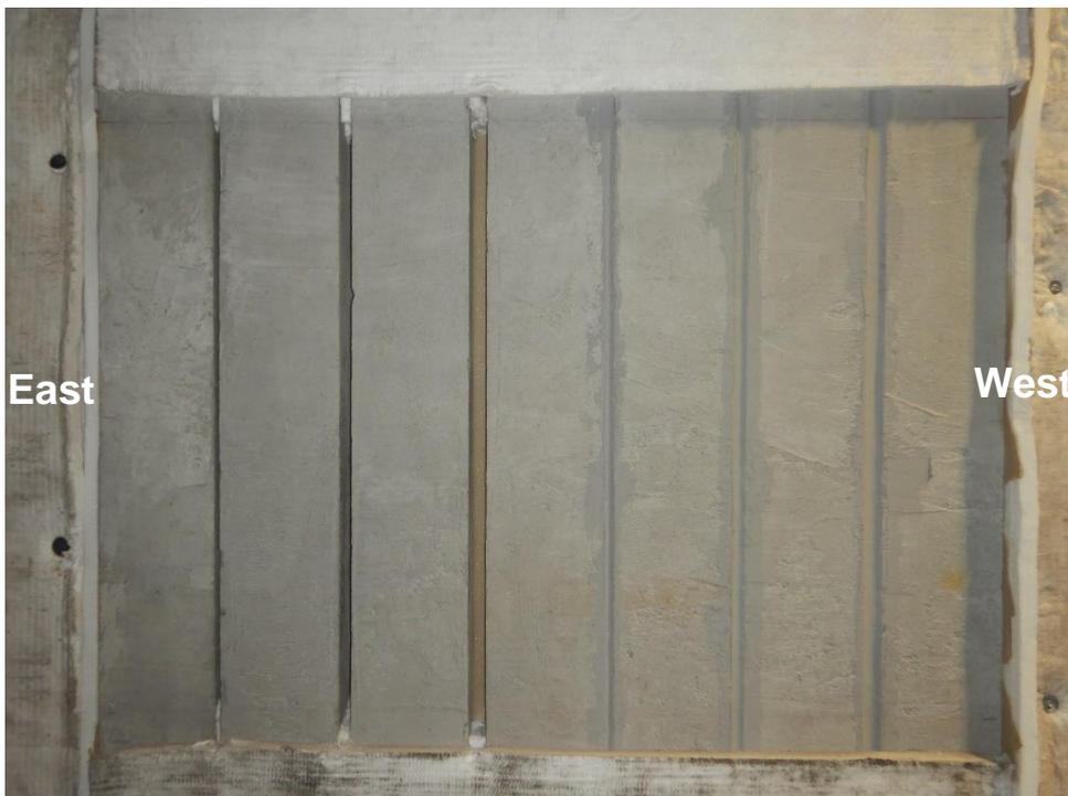
Figure 24 Exposed face of the specimen before the start of the fire-resistance test
