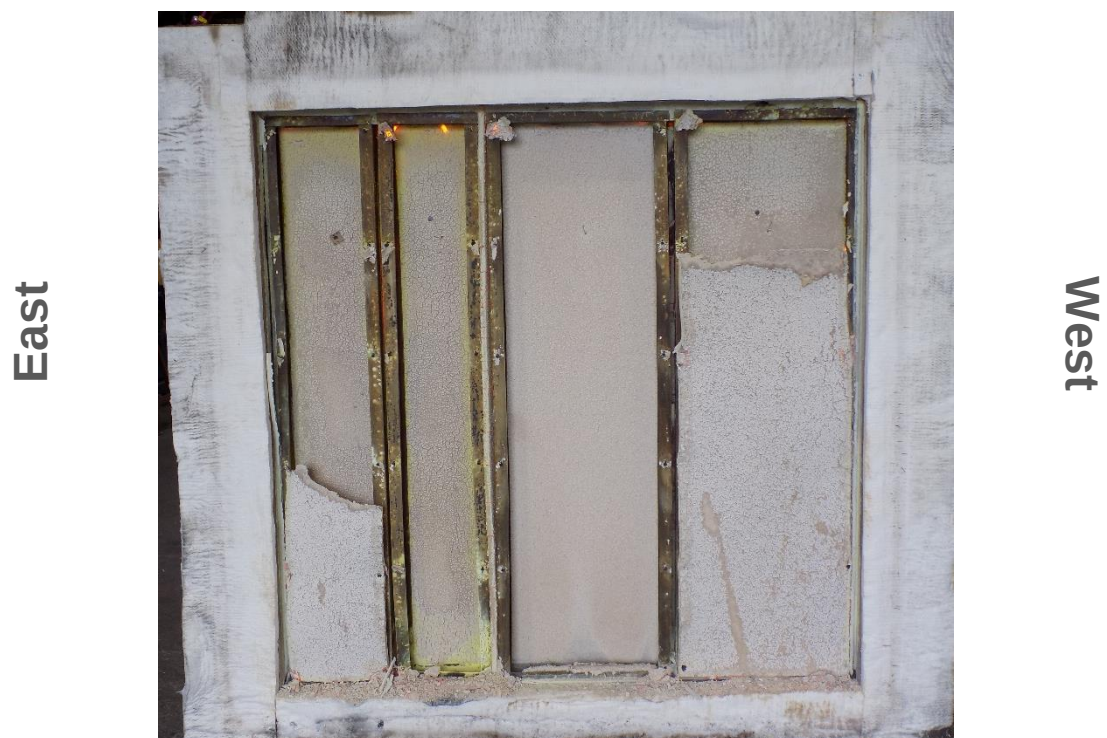
Figure 19 Exposed face of the specimen at the end of test
