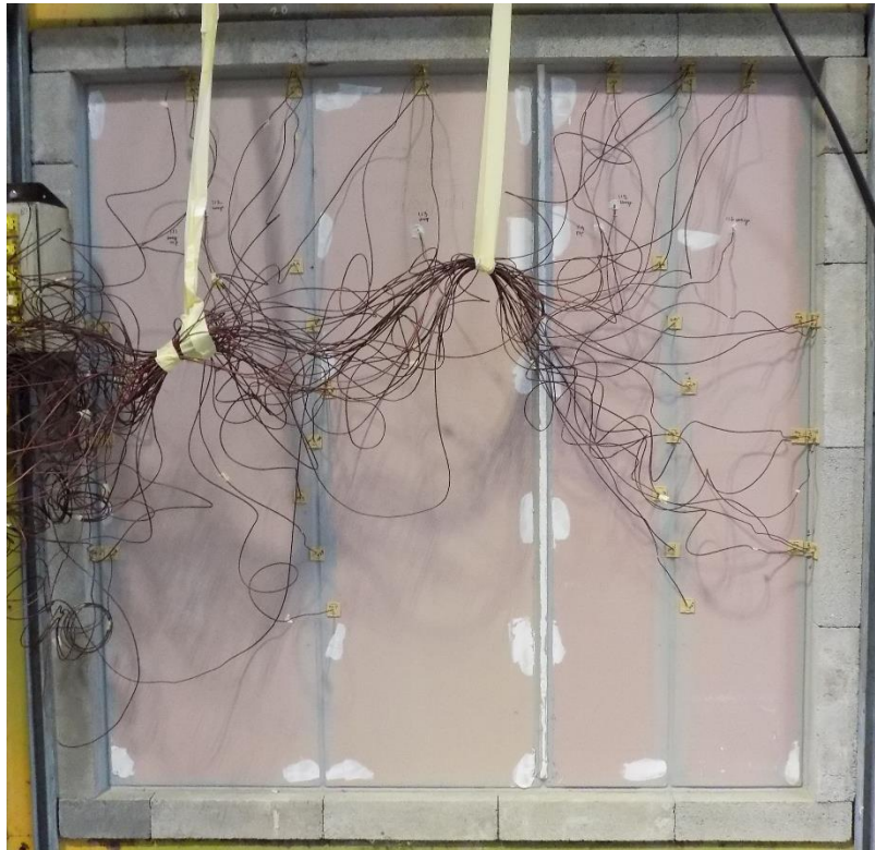
Figure 16 Unexposed face of specimen before the start of test
