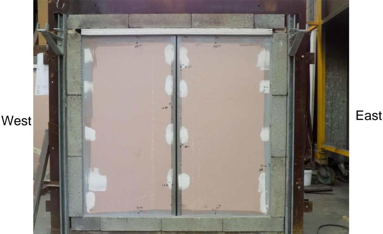
Figure A6.1: Unexposed face of specimen before commencement of the fire-resistance test
