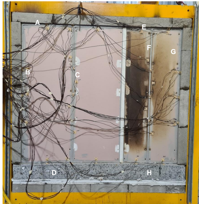
Figure 18 Unexposed face of the specimen at the end of the test
