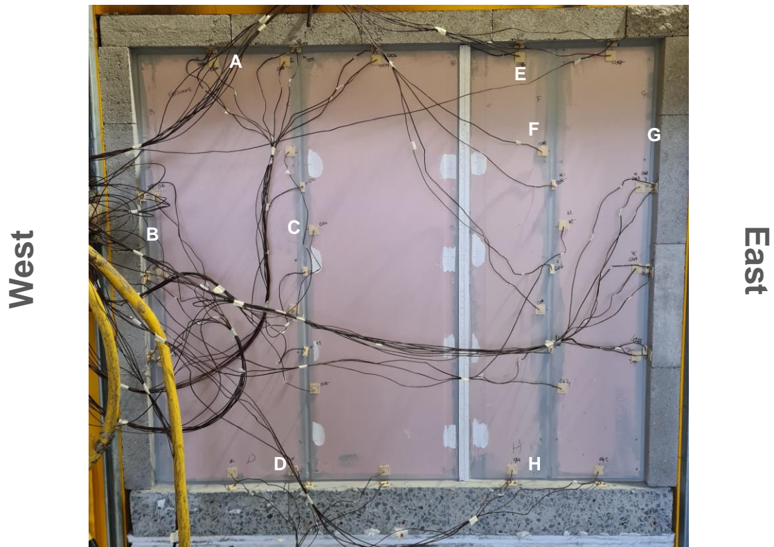
Figure 16 Unexposed face of the specimen before the start of the test
