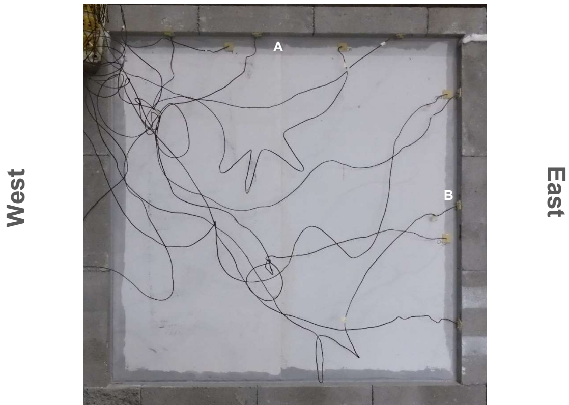
Figure 14 Unexposed face of the specimen before the start of the test
