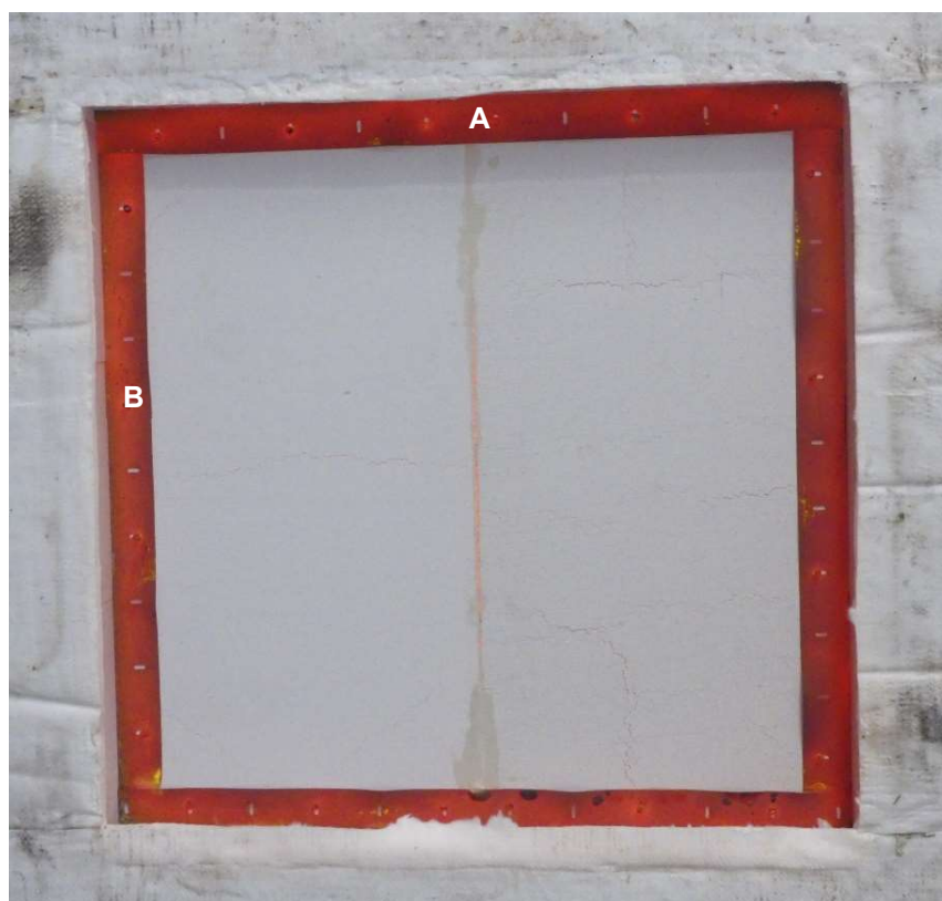
Figure 17 Exposed face of the specimen at the end of the test
