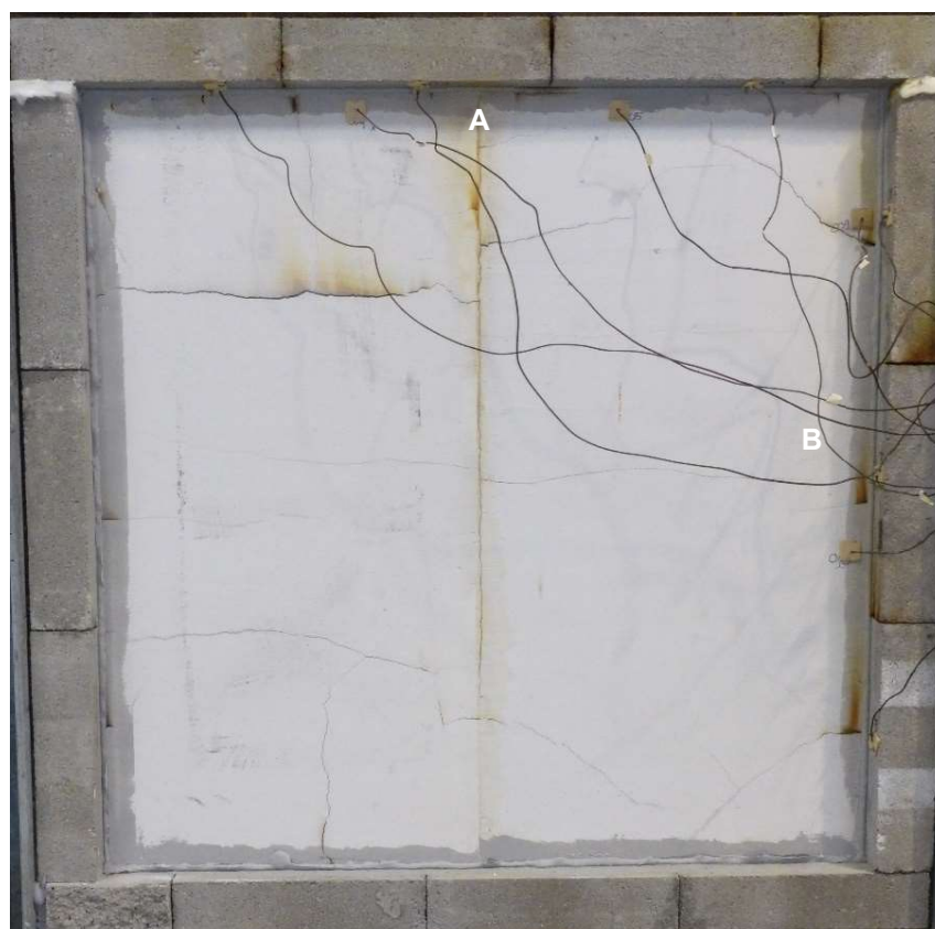
Figure 16 Unexposed face of the specimen at the end of the test
