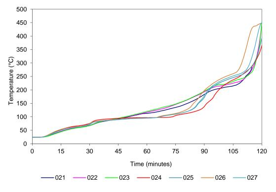
Figure 9 Penetration system B – temperature vs time
