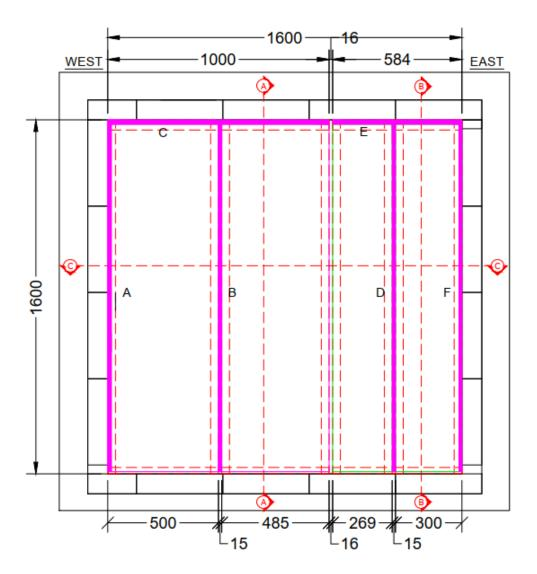
Figure 1 Elevation view of test specimen (unexposed side)
