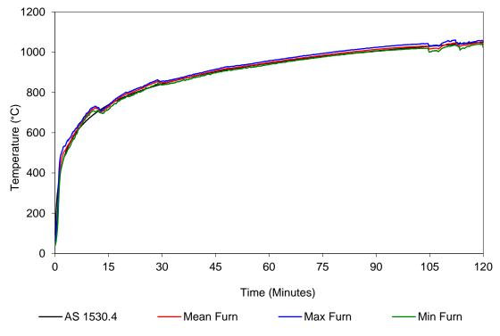
Figure 7 Furnace thermocouple temperature vs time
