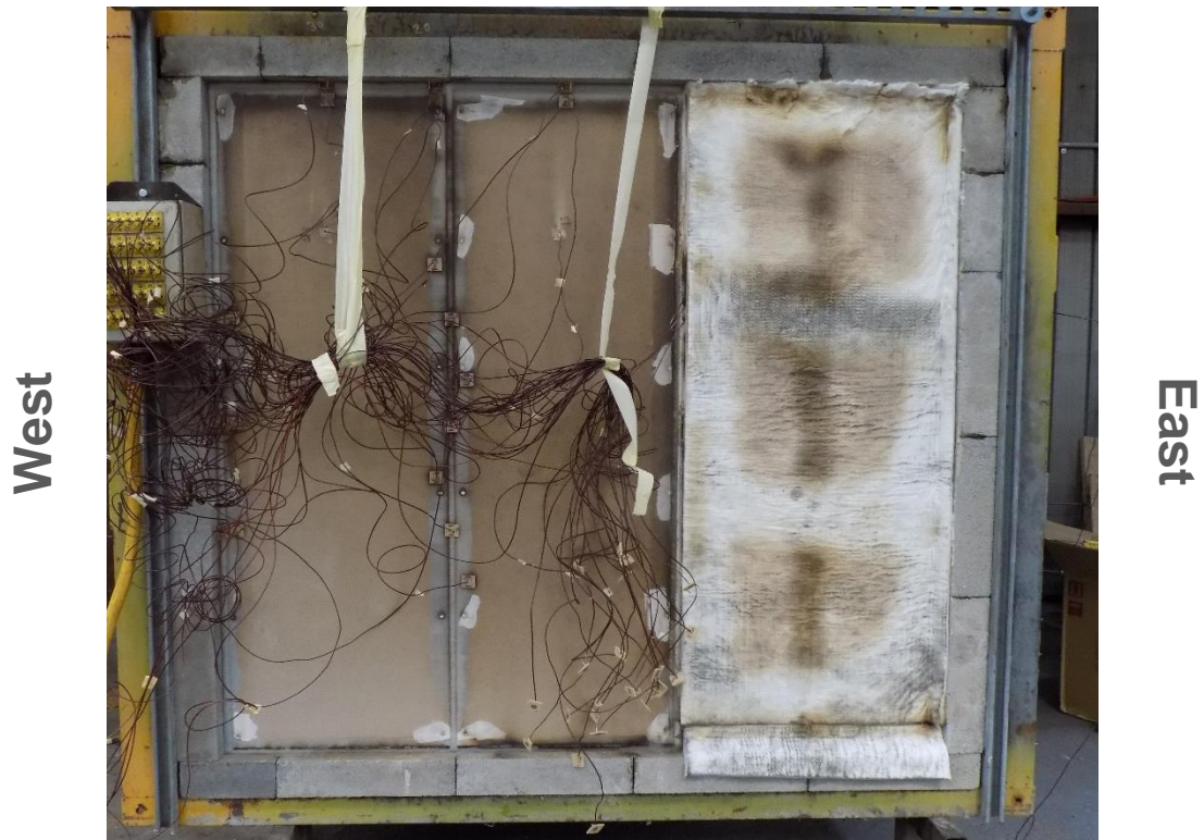
Figure 18 Unexposed face of specimen at the end of test
