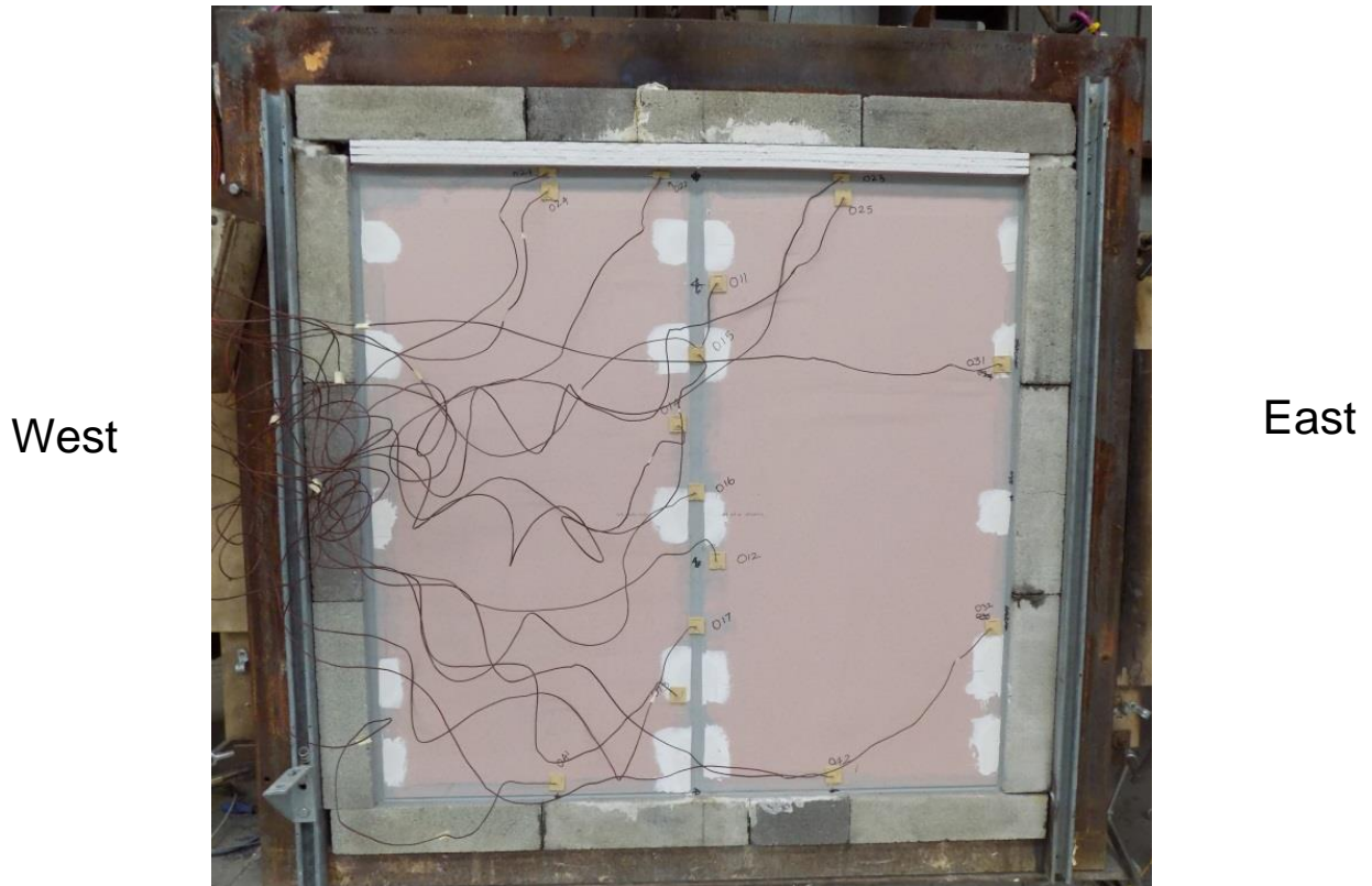
Figure A6.1: Unexposed face of specimen before commencement of the fire-resistance test
