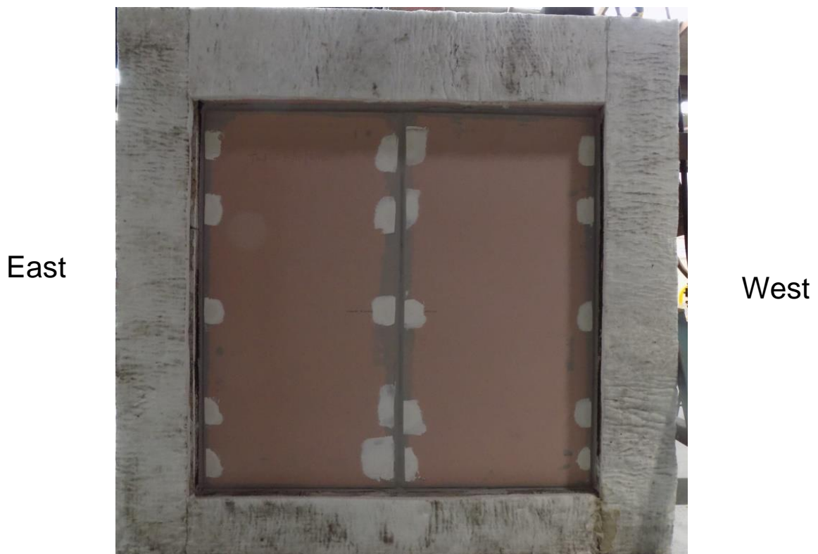
Figure A6.2: Exposed face of specimen before commencement of the fire-resistance test
