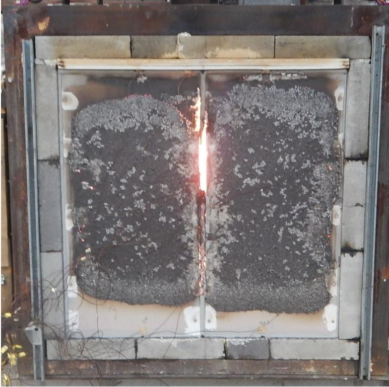
Figure A6.3: Unexposed face of specimen at the end of the test.
