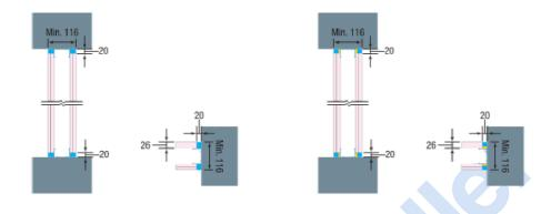
2 x 13mm Plasterboard - Perimeter Joints (Horizontal + Vertical)
