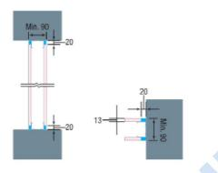
1 x 16mm Plasterboard Perimeter Joints (Horizontal + Vertical)
