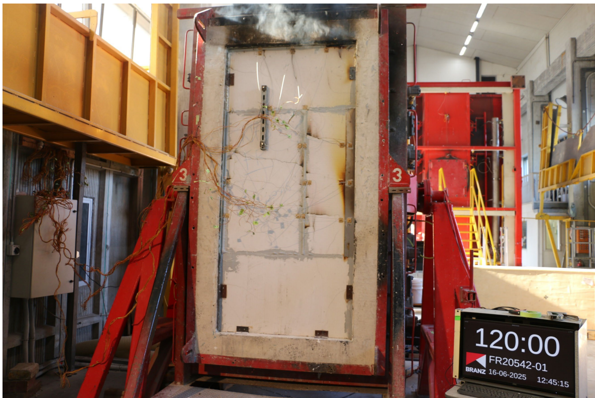
Photo 6: The Unexposed Face of the Test Assembly After a Duration of 132 Minutes
