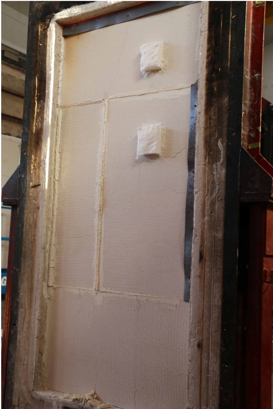
Photo 7: The Exposed Face of the Test Assembly Immediately After Testing
