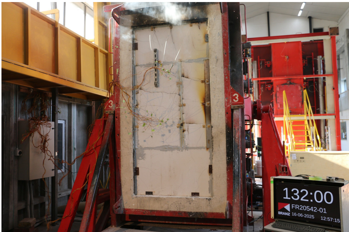
Photo 6: The Unexposed Face of the Test Assembly After a Duration of 132 Minutes
