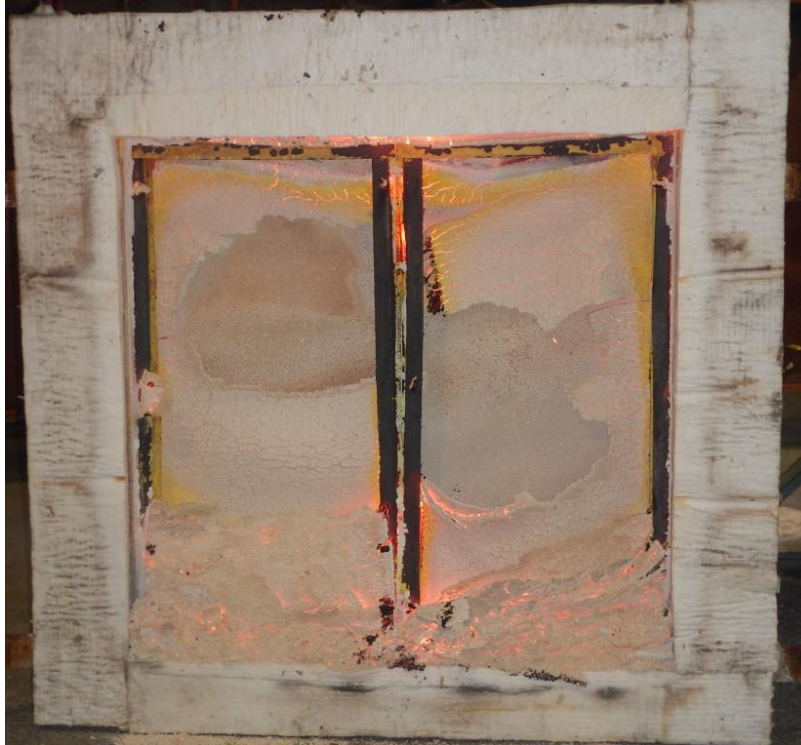
Figure 20 Exposed face of the specimen at the end of the test
