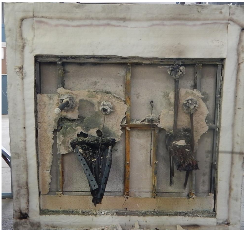
Figure 31 Exposed face of the specimen at the end of the test
