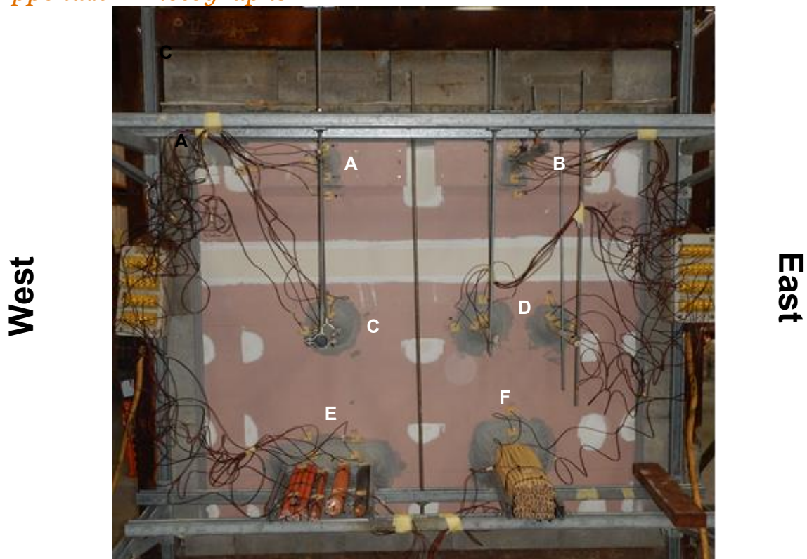
Figure 29 Unexposed face of the specimen before the start of the test
