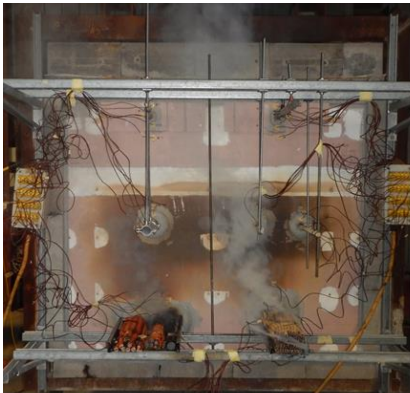
Figure 31 Unexposed face of the specimen at the end of the test
