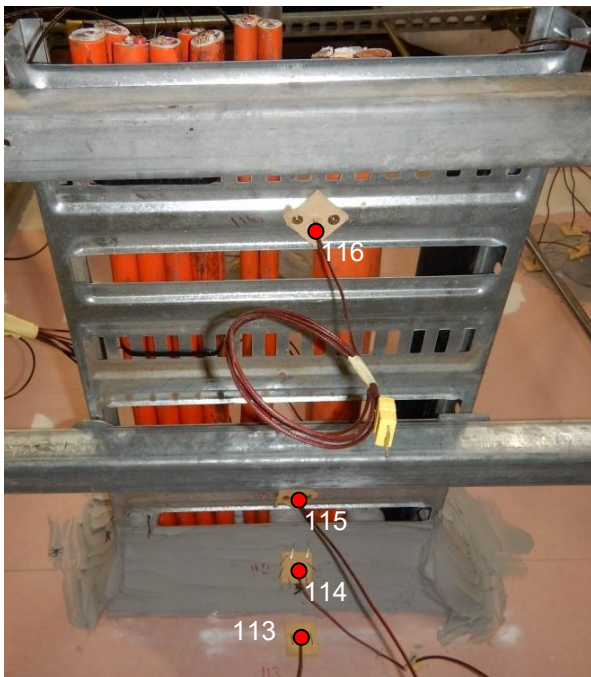
Figure 12 Penetration system E bottom
