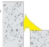
Incorrect: No backing rod used. Too much sealant in joint (not concave). Too much sealant adhering to substrates.
