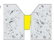
Incorrect: No backing rod, poor sealant depth/width ratio, too much sealant adhering to substrate
