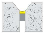
Incorrect: Incorrect joint depth/width ratio
