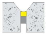
Correct: Correct depth/width ratio, correct amount of sealant adhering to substrate, acceptable backing rod application, tooling of sealant creating acceptable joint top surface
