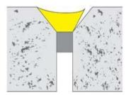
Incorrect: Incorrect sealant depth/width ratio and joint dimension, too much sealant adhering to substrate
