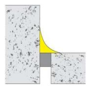
Correct: Backing rod used correctly. Correct amount of sealant in joint (slightly concave). Correct amount of sealant adhering to substrate.
