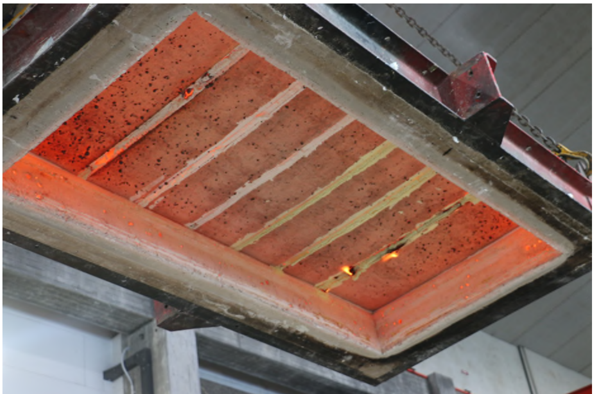
Photo 6: The Exposed Face of the Test Assembly Immediately After Testing
