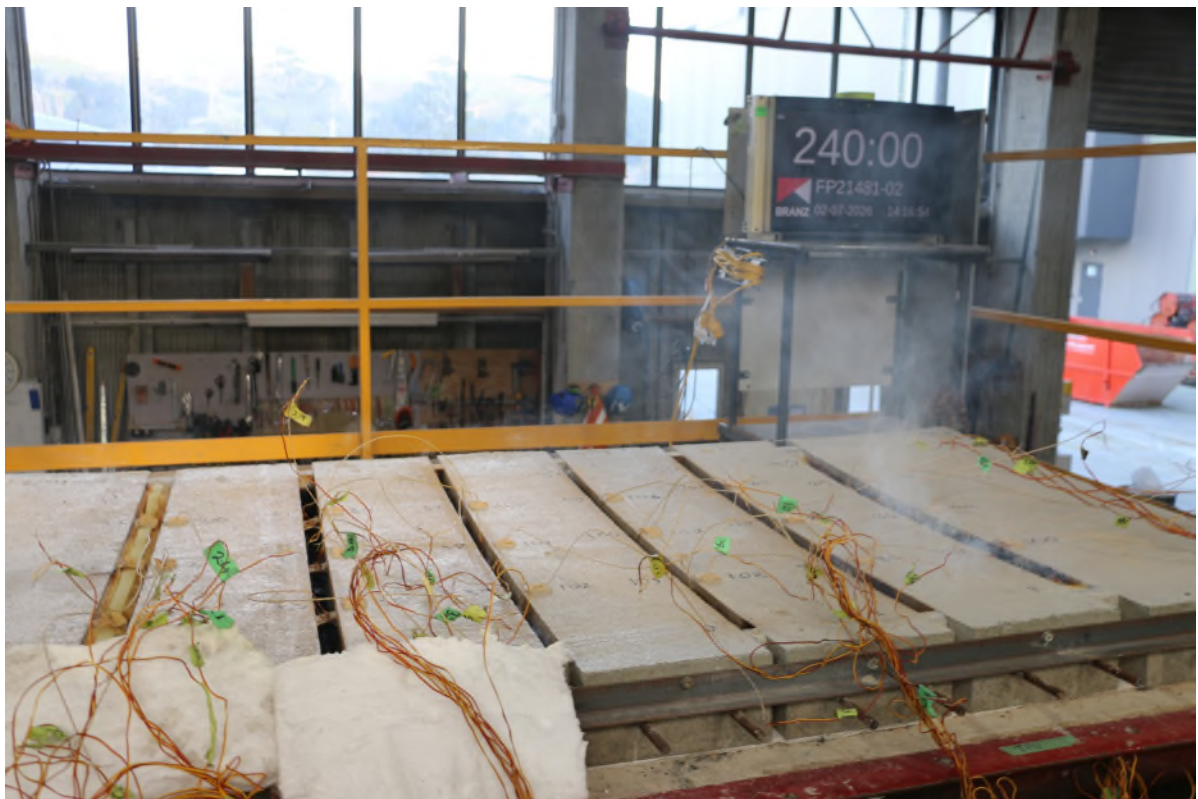
Photo 6: The Exposed Face of the Test Assembly Immediately After Testing
